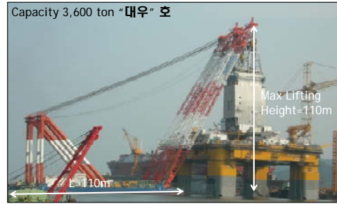
Fig. 7 Configuration of the 3,600 ton floating crane (Cha 2008)
