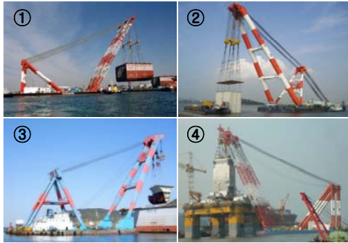
Fig. 1 Examples of Various operations of floating cranes (①, ②, ③: Erection of mega blocks, ④: Lifting derrick)
