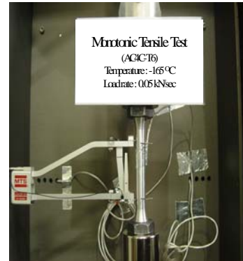
Fig. 3 Experimental configuration of monotonic tensile test
