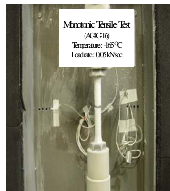
Fig. 4 Fractured specimen after monotonic tensile test
