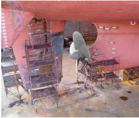
Fig. 1 Typical profile of the rudder erosion
