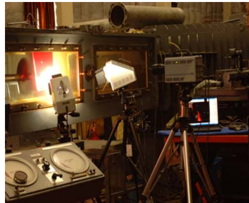
Fig. 14 Experimental set-up for cavitation test
