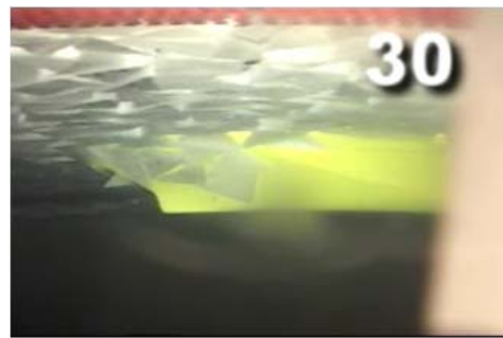
Fig. 17 Under water view of resistance test with thin pack ice (0.4m/s, 90%, \phi = 30^\circ )
