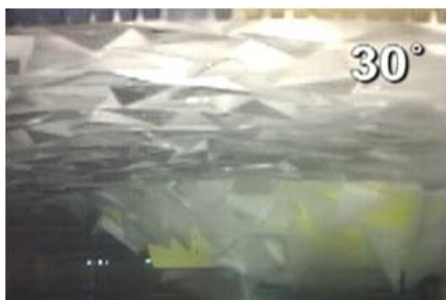
Fig. 11 Under water view of resistance test with thick pack ice (0.4m/s, 90%, \phi = 30^\circ )
