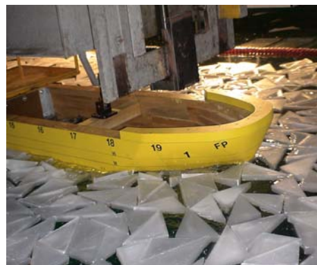
Fig. 5 Profile of resistance test with synthetic ice
