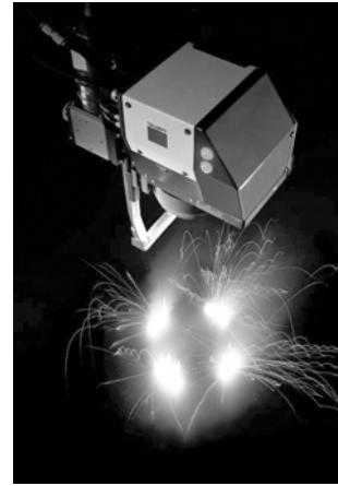
Fig. 11 Remote welding with a TRUMPF programmable focusing optics (PFO)
