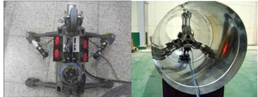
Fig. 15 Test of the in-pipe robot
