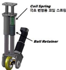
Fig. 2 Module of the compressible spring
