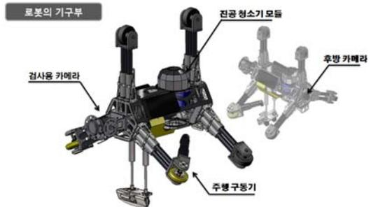
Fig. 1 Design of the in-pipe robot
