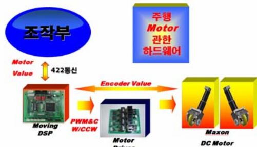
Fig. 7 Control structure of the driving motors
