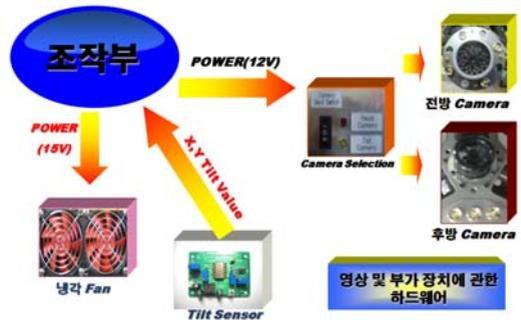
Fig. 10 Control structure of the camera and the sensor
