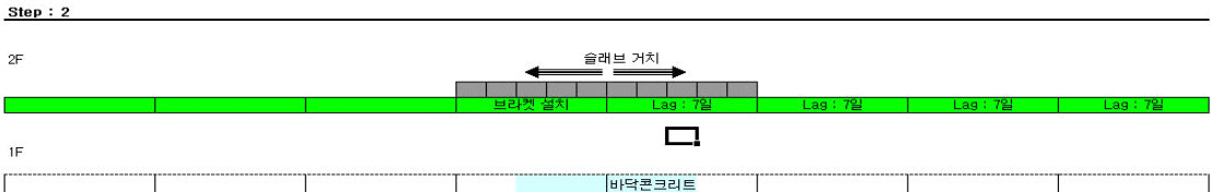
(b) 2nd Stage: Construction of Bridge Road and Base Concrete
