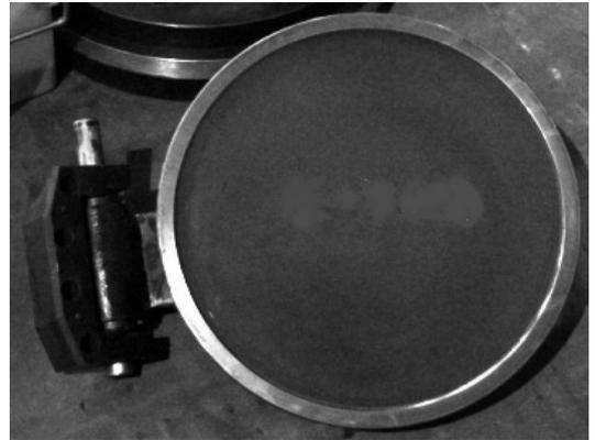
Fig. 2 Swing check valve disk and hinge
