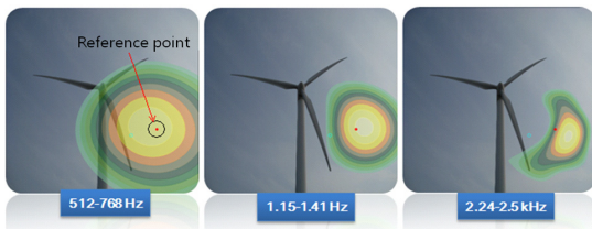
Fig. 4 The localized noise source about the function of band frequency( \alpha=46^\circ )
