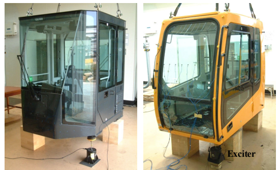
Fig. 7 Experimental setup for structureborne noise
