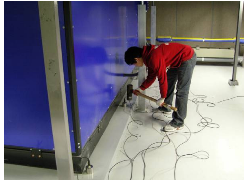
(a) Loading by impact hammer
