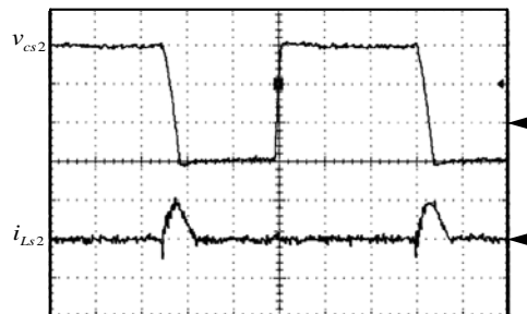
Fig. 10. Experimental waveforms : v_{cs2} (100 V/div) and i_{Ls2} (1 A/div), time: 5 \mu s /div.
