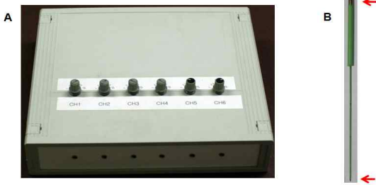
Fig. 1. A prototype of high frequency warm needling device (A) and teflon coated stainless steel acupuncture needle (B). Arrows indicate un-coated regions which is needle tip (1mm) and top of needle (3mm) connected to device.
