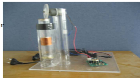
Fig. 5. Vibration power generation experimental device
