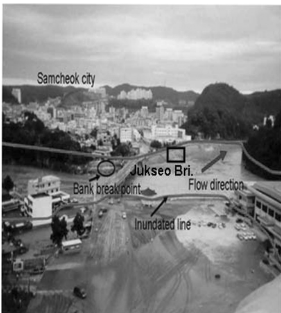
Fig. 1 Inundated situation of study area during the flooding of 2002 (□: outlet of sewer line)
