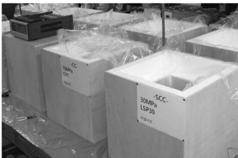
Fig. 1 Semi adiabatic temperature apparatus of concrete
