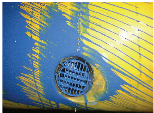
Fig. 2 Paint test result of 138K LNGC with bow thruster (tunnel with scallop, grid and CPP).
