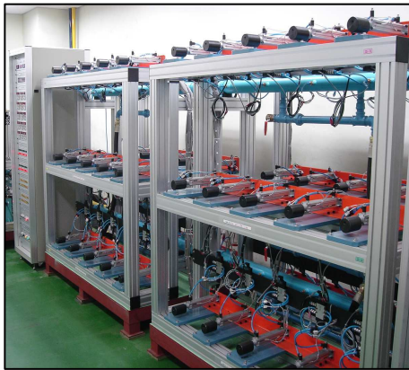
Fig. 2 Life Tester of Pneumatic Cylinder
