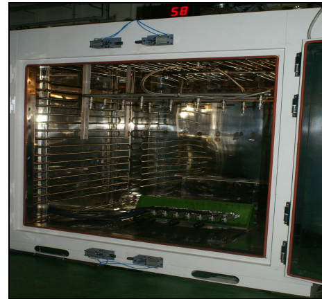
Fig. 3 Environment Chamber for the Accelerated Life Test
