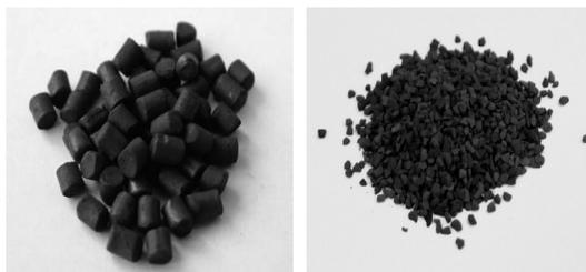
Fig. 2  $\text{MnO}_2/\text{Al}_2\text{O}_3$  samples (1/8", 16-20 mesh)
