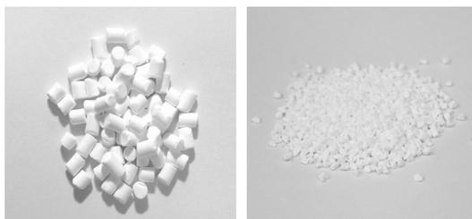
Fig. 1 Alumina pellet samples (1/8", 16-20 mesh)
