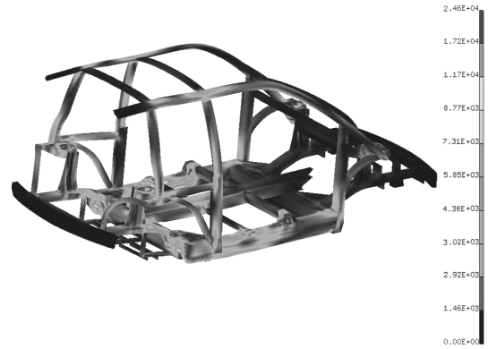
Fig. 5 Sum of scaled kinetic energy from 1st to 5th mode
