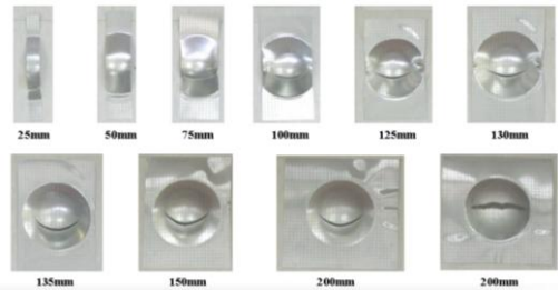
Fig. 6 Specimens after the formability test
