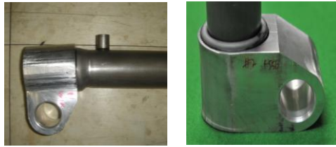
(a) bending failure (b) buckling failure
