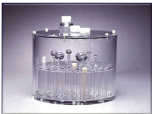
Fig. 2. Flangeless Esser PET Phantom.
