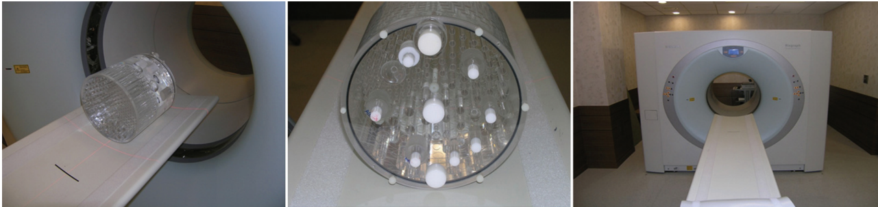
Fig. 1. Data spectrum corporation flangeless esser PET phantom TM and siemens biograph 40 true-point.
