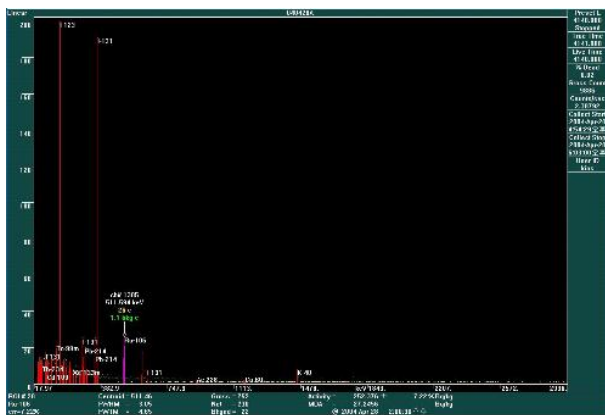
Fig. 1. Gamma Spectroscopy of Korean Nuclear Medicine Worker's Urine: Iodine ( ^{123}\text{I} , ^{131}\text{I} ) Peak.
