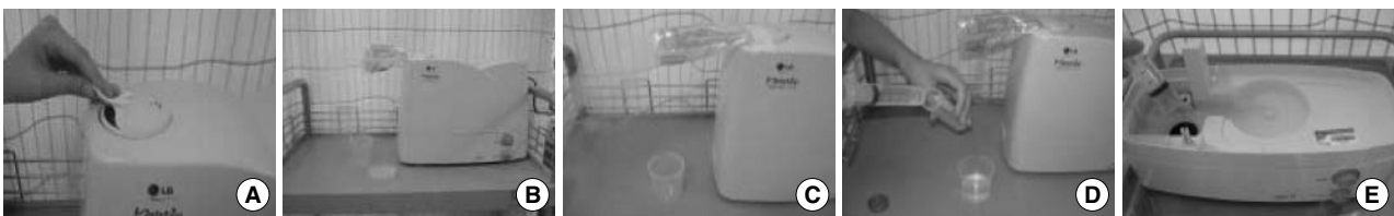
Fig. 2. Waterdrop sampling from the outlet of humidifier. (A) Rub outlet of humidifier with alcohol cotton. (B) Cover outlet of humidifier with aseptically bag and fix the bag. (C) Collect waterdrop from the bag with aseptically collecting tube. (D) Sample 50 cc waterdrop into the collecting tube with syringes. (E) Sample 50 cc water around oscillating body with syringes.
