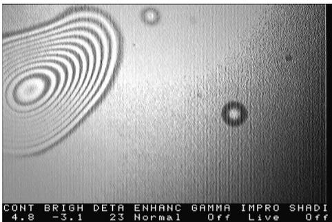
Fig. 7 Result of bonded wafer void an- alysis by laser
