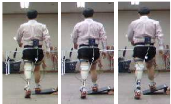
Fig. 5 Custom-made slop(up, 5, 10, 15 degrees) and 19 reflective markers were used in motion analysis (down)
