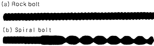
Fig. 1. Appearance of rock and spiral bolts.
