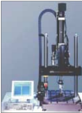
Fig. 3. Instron 8871 Dynamic Material Testing Machine (Instron, UK) 8871: Axial-only. Maximum load capacities of \pm 5 KN ( \pm 1.1 Kip) and \pm 10 KN ( \pm 2.2 Kip).
