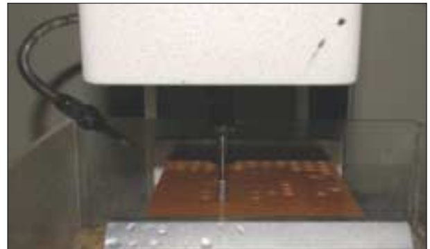
Fig. 2. Forming of insertion hole with auto drilling machine.
