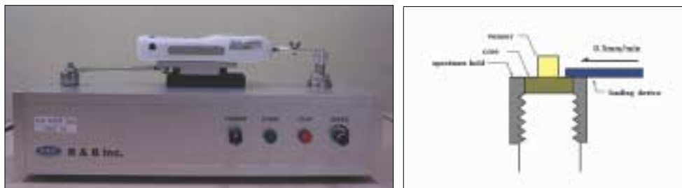
Fig. 2. Shear bond test machine (Simple Tensile Tester Model No. RB312 PETI, R&B Inc., Daejeon, Korea).
