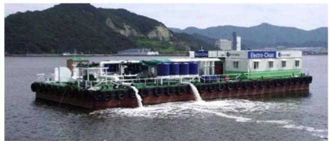
Fig. 2. Testing Barge for Land-Based Test.
