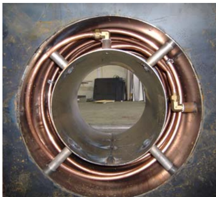
Fig. 6. PCM storage part.
