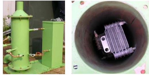
Fig. 3. Heat exchanger using waste gas.
