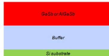
Fig. 7. Epi structure used for recess etching
