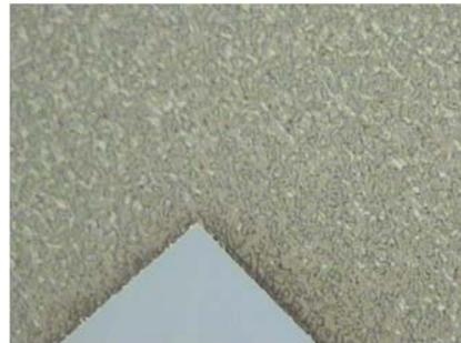
Fig. 4. HF-based etching surface (after 1 min etching)
