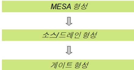
Fig. 1. HEMT device process flow
