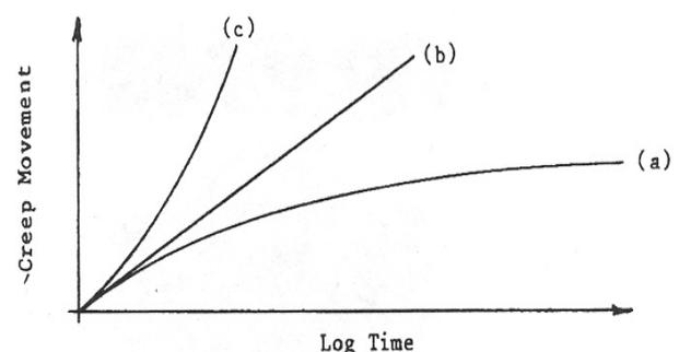
Fig. 10. Creep characteristic curves (Weatherby, 1982)
