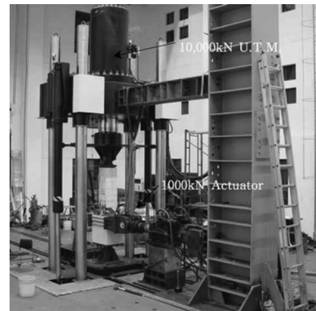
Fig. 2 Set-up of specimen
