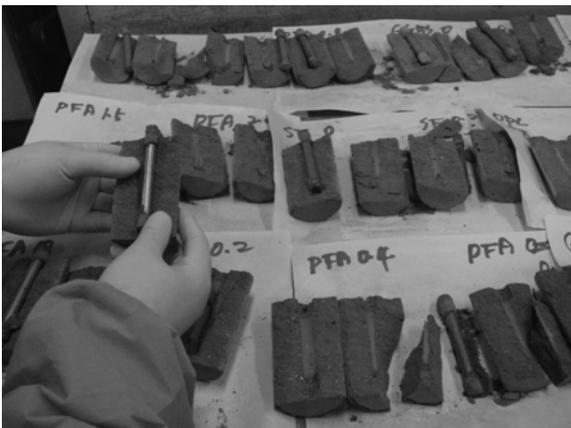
Fig. 8 Visual inspection after corrosion monitoring
