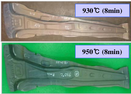
Fig. 4 Al-Si coated steel after heating test
