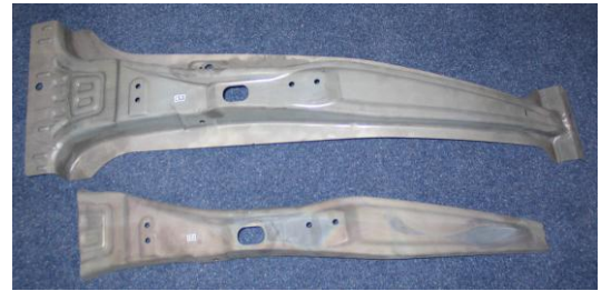
Fig. 6 Appearance of hot-stamping center-pillar
