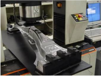
Fig.11 Test jig for compression test (30ton UTM)
