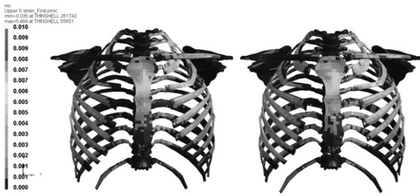
Fig. 12 Strain contour comparison of 0.5m/s belt loading case
