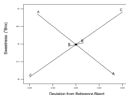
Fig. 4. Response surface and trace plot for the effect of paste (A), pectin (B), and sugar (C) on sweetness (°Brix) of Chinese quince jam.
