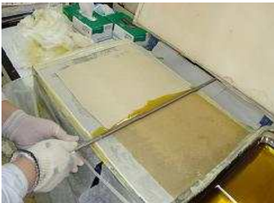
Fig. 1. Brushing method by using heating dryer and coating bar.
