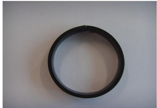
Figure 3. Picture of circularly deformed rubber sample.
