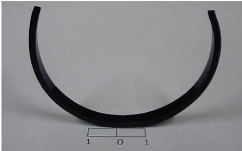
**Figure 4.** Picture of the deformed rubber sample after release following thermal aging under circular deformation.
