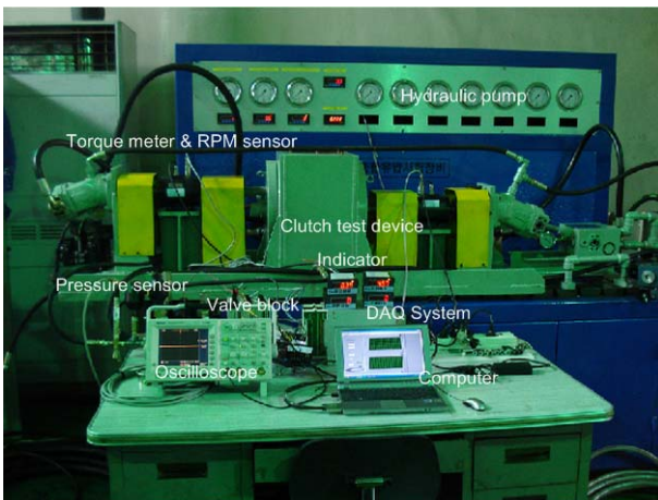
Fig. 10 Test rig for power-shift clutch test
