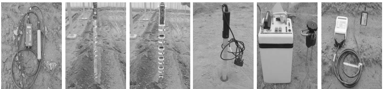
Fig. 1. Sensors tested in the experiment (TRIME, EasyAG, EnviroSCAN, PR-1, Mini-TRASE, and WET-1 from the left).
