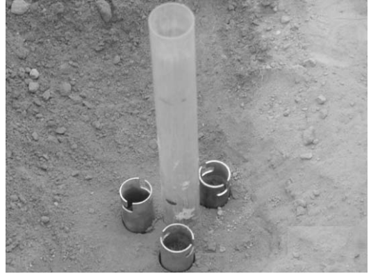
Fig. 2. Soil sampling by core for volumetric soil water content.
