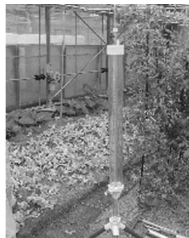
Fig 2. Guelph permeameter (GPM).
