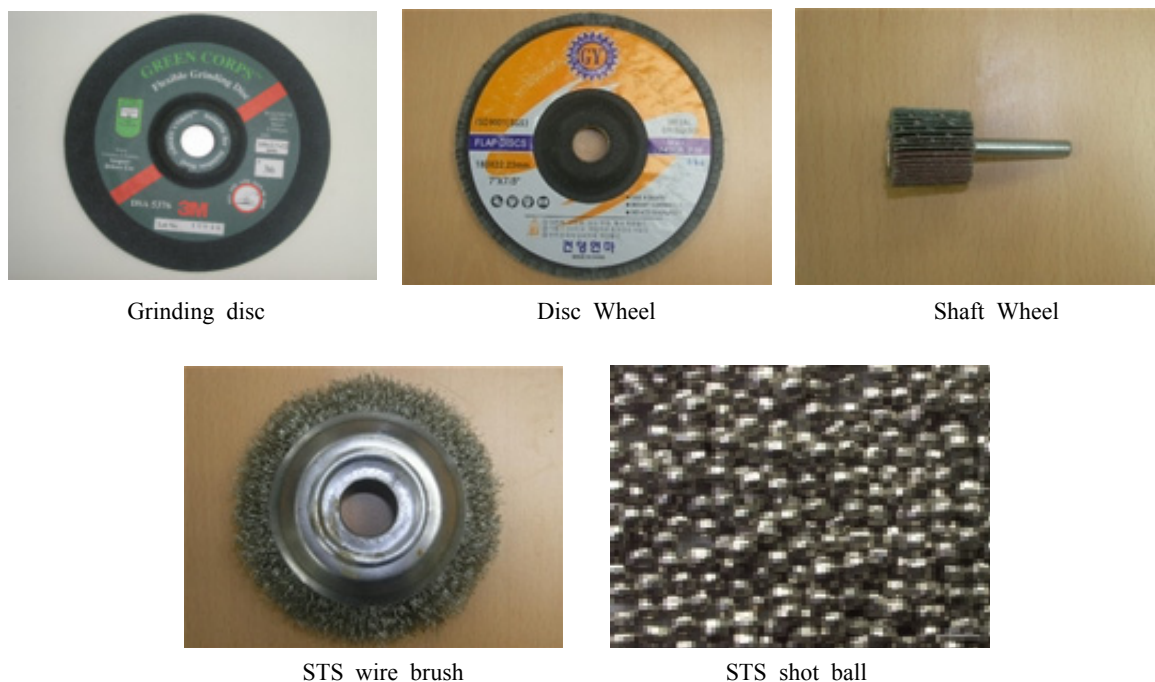
Fig. 1. Different tools used for mechanical surface treatment methods.
