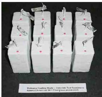
Fig. 1. Completion of base Coating
