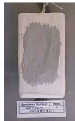
Fig. 3. overlapping of repair coating
