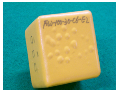
Fig. 1. Osmotic blistering of coating on concrete
