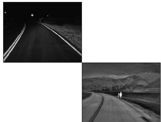
Fig. 2 Comparison of visible light and thermal infrared
