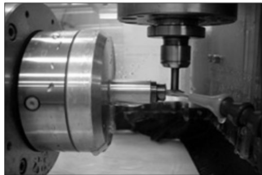
Fig. 15 Aspheric processing scene
